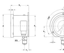
A + C surface mounting, back flange; lower connection.
